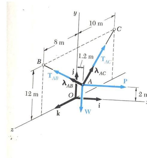
$$\begin{aligned} W &= -mg \vec{j} = -(200 \text{ kg})(9.81 \text{ m/s}^2) \vec{j} \\ &= -1962 \text{ N} \vec{j} \\ P &= P \vec{i} \end{aligned}$$
