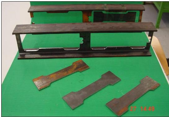
Figure 7: Samples location and specimens geometry.
