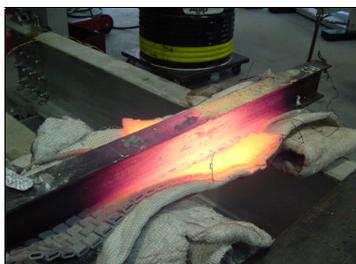
Figure 5: Beam heated at 800 [°C] during one hour.
