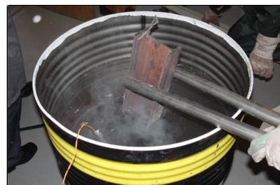
Figure 6: Beam cooling procedure (quenching).
